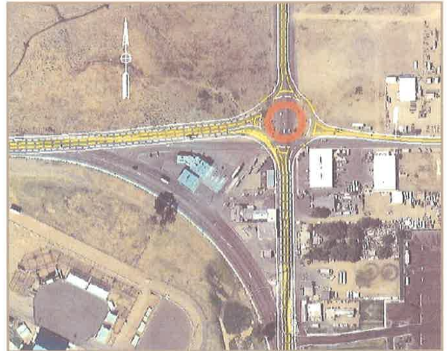
Figure 2-4, "Wye" Intersection Reconfiguration Alternative
