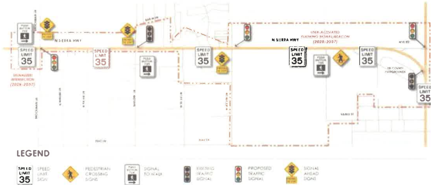
Figure 2-18 Long-Term Implementation Traffic Controls
