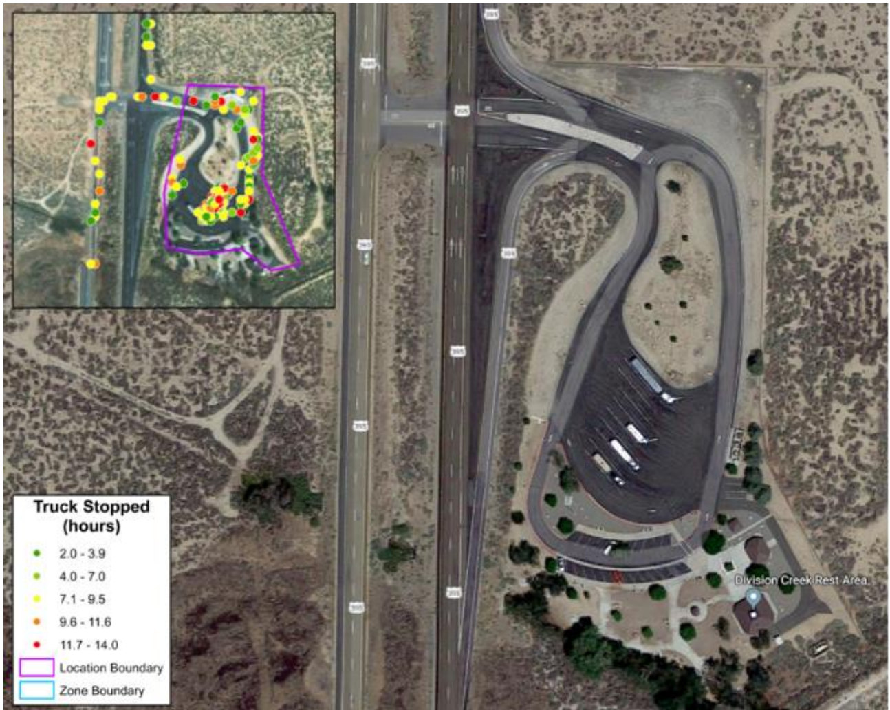
Figure 9.4 Truck Parking Demand at Division Creek Rest Area
