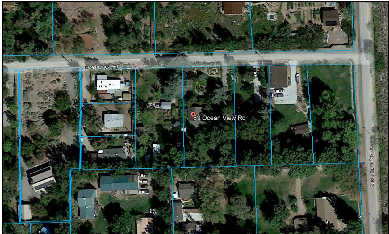
Figure D.10. 53 Ocean View Rd property. Structures have poor defensible space, with some branches resting on the roof. Wooden deck and fence in the southwest corner are connected to vegetation. The property is accessible only via Ocean View Rd. The blue boundary is the parcel boundary.
