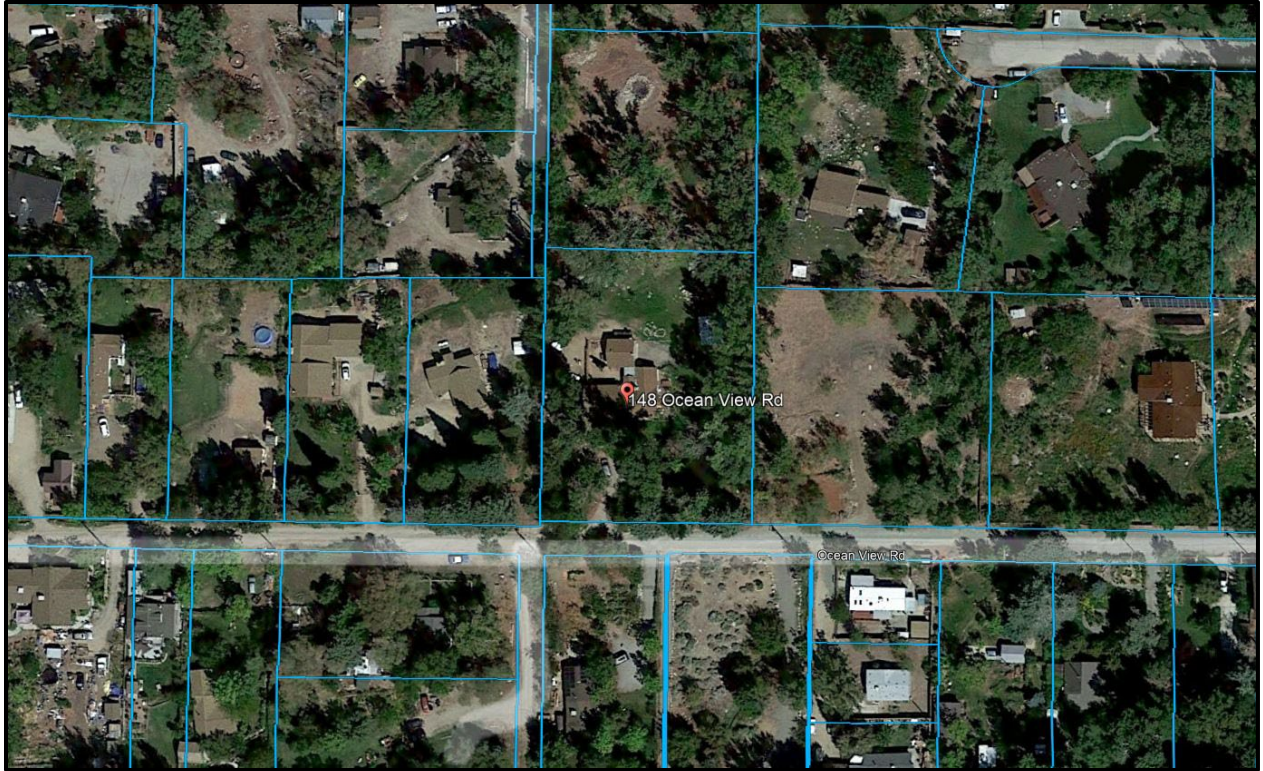
Figure D.11. 148 Ocean View Rd property. Structures have limited defensible space, with some branches contacting roofs. The property is accessible only via Ocean View Rd. The blue boundary is the parcel boundary.
