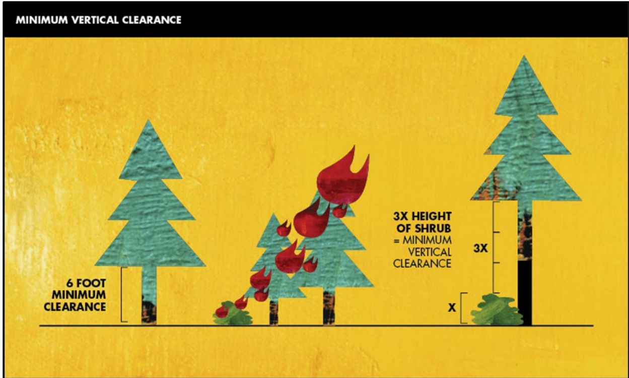
Figure J.4. Minimum vertical clearance.
