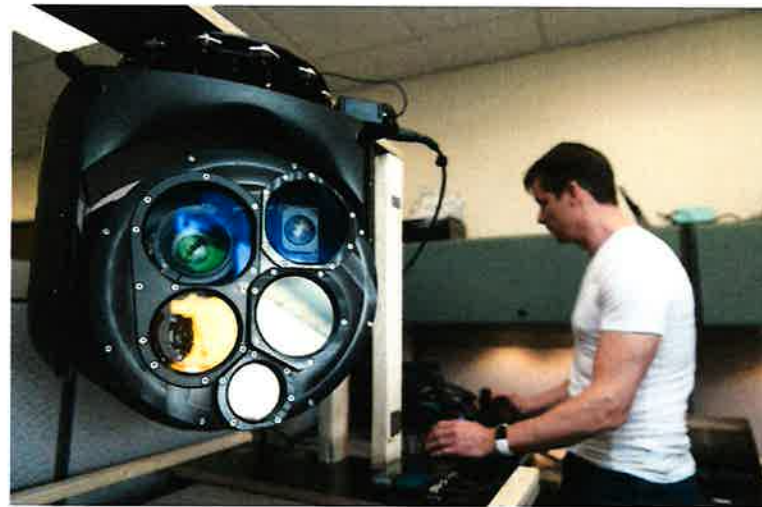
SCE's helicopters are equipped with software and high-tech cameras, like the one shown above, to find potential risk undetectable to the human eye
