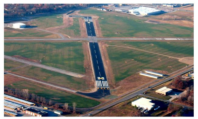
Figure 2-3. Markings for a Temporarily Closed Runway
