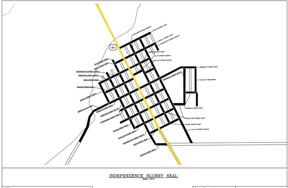
BLACKENED Roads are the roads that are getting slurry seal. LEGEND: : SLURRY SEAL
