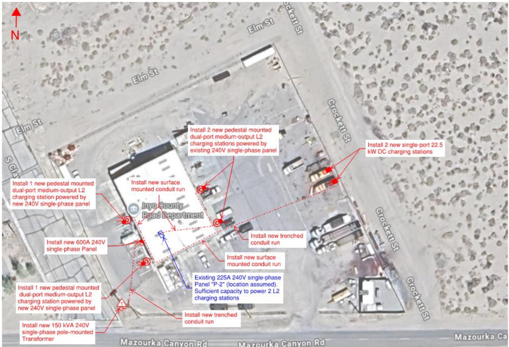
FIGURE 57: MAZOURKA ROAD YARD CONCEPTUAL DRAWING PROPOSED EVSE
