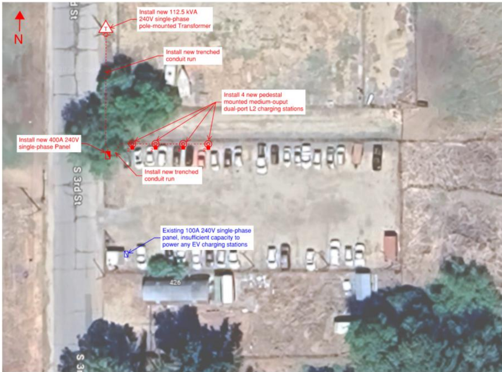
FIGURE 52: 3RD STREET YARD CONCEPTUAL DRAWING PROPOSED EVSE
