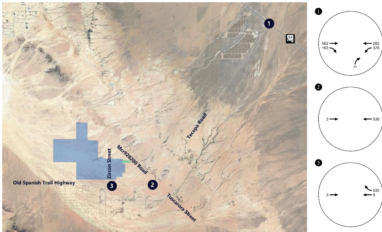
Figure 6: AM Peak Hour Intersection Volumes During Project Construction
