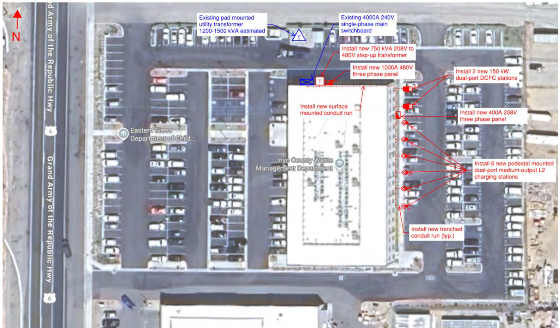
FIGURE 51: COB CONCEPTUAL DRAWING FOR PROPOSED EVSE
