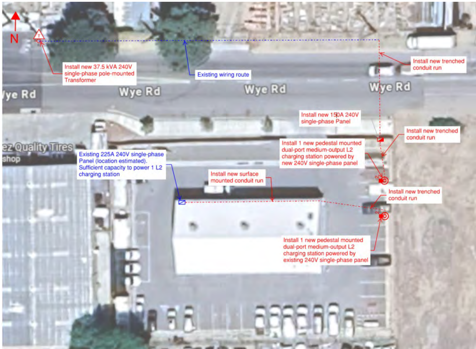
FIGURE 59: WYE ROAD CONCEPTUAL DRAWING PROPOSED EVSE
