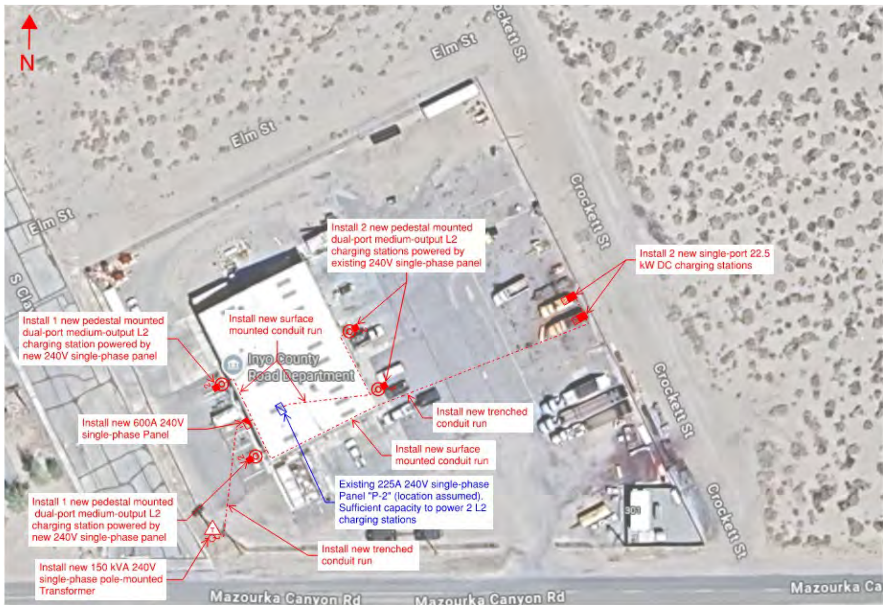
FIGURE 57: MAZOURKA ROAD YARD CONCEPTUAL DRAWING PROPOSED EVSE
