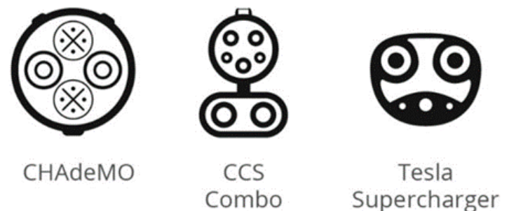
FIGURE 5: DCFC CONNECTOR TYPES
