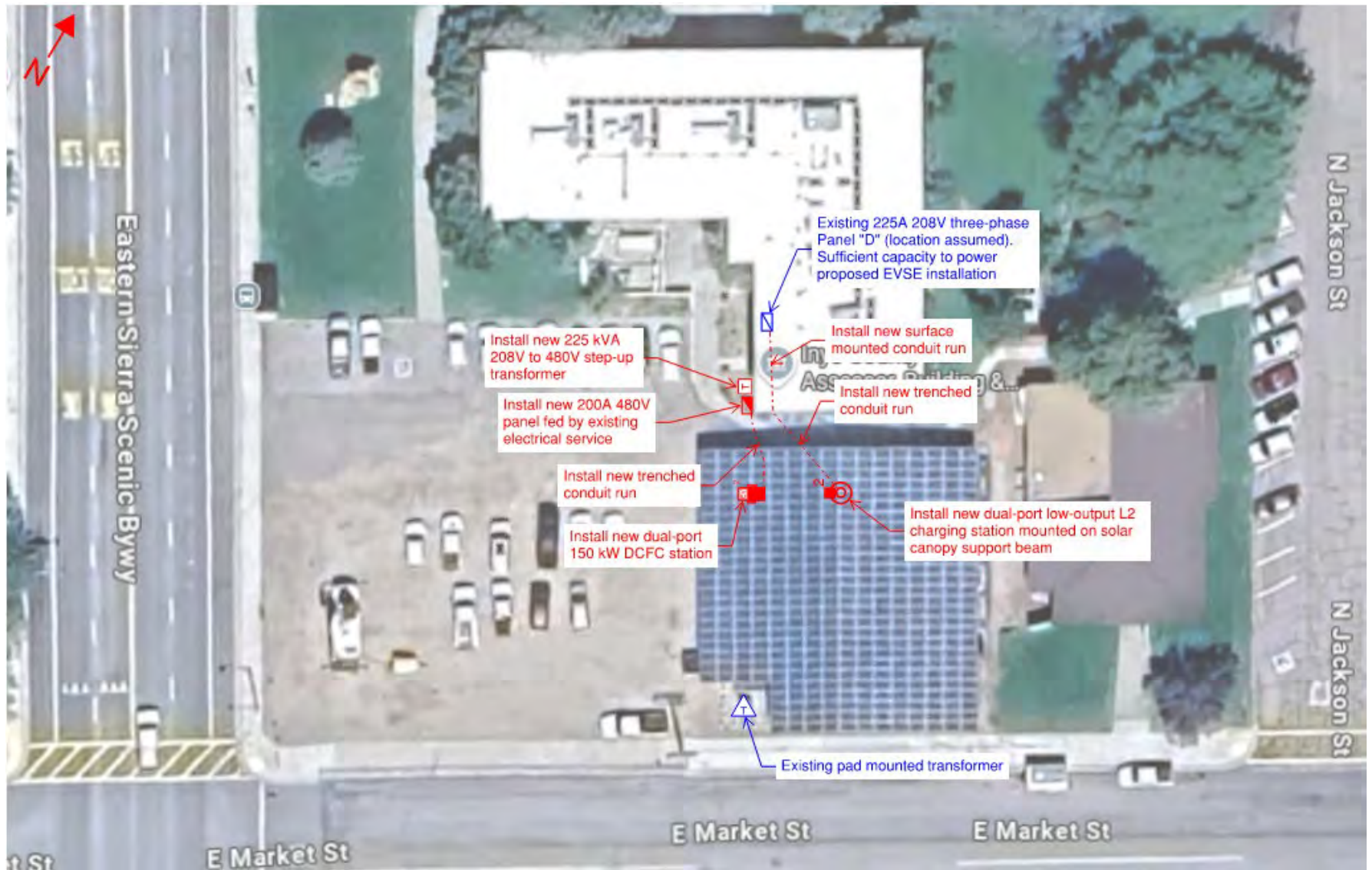
FIGURE 55: INYO COUNTY ANNEX CONCEPTUAL DRAWING PROPOSED EVSE
