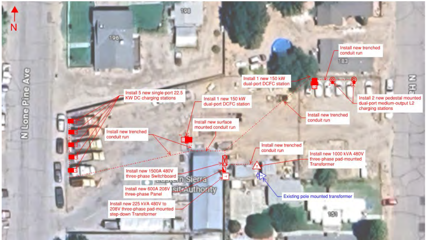
FIGURE 56: LONE PINE YARD CONCEPTUAL DRAWING PROPOSED EVSE
