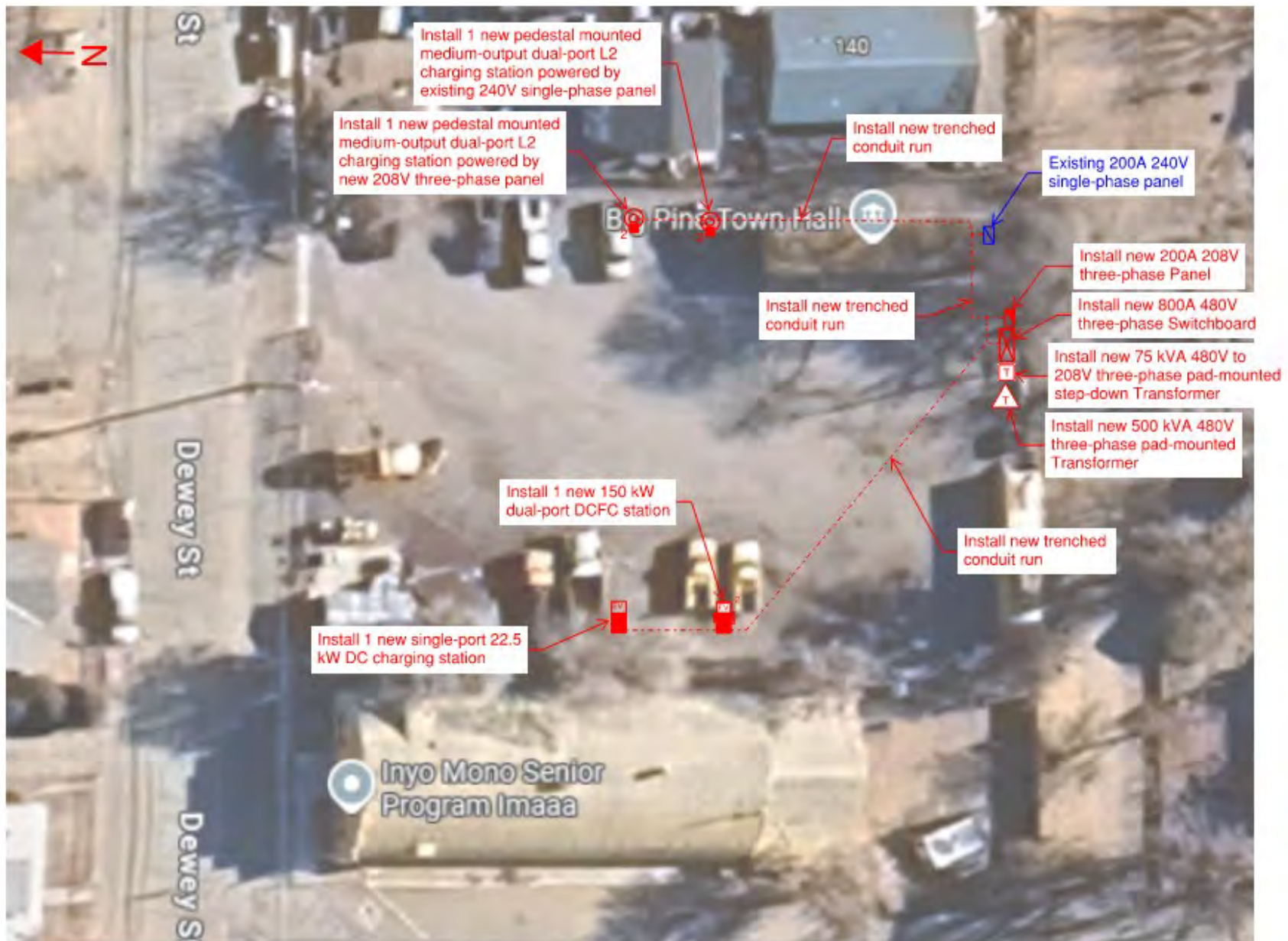
FIGURE 53: BIG PINE ROAD YARD CONCEPTUAL DRAWING PROPOSED EVSE
