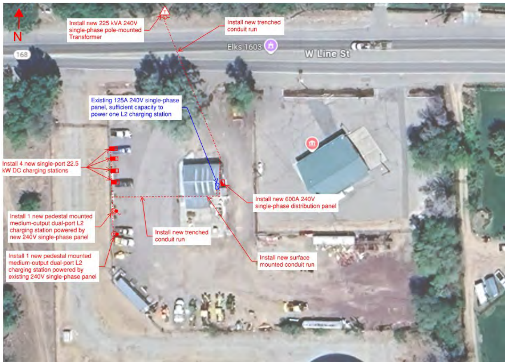
FIGURE 54: BISHOP ROAD YARD CONCEPTUAL DRAWING PROPOSED EVSE
